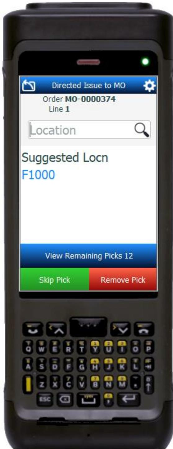
This application allows the user to enter multiple manufacturing orders and uses the system to logically group parts by location and then directs the user around the warehouse to pick and associate the parts to their individual MO.
