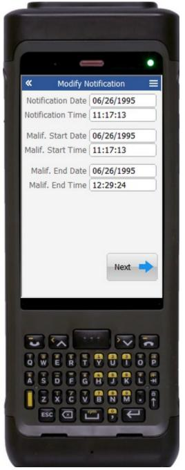
The second page contains optional values for when the notification was created, when the malfunction started, and when the malfunction was corrected.
